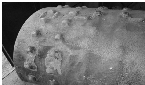
Fig. 3. Rolling crusher with worn teeth and teeth reconditioned
