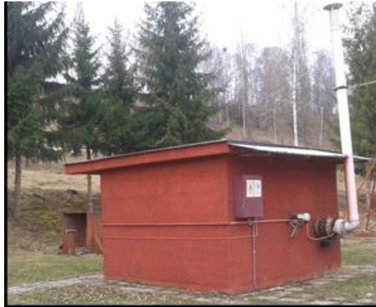
Fig. 5 Armoured explosion chamber for the determination of explosion toxic gases
