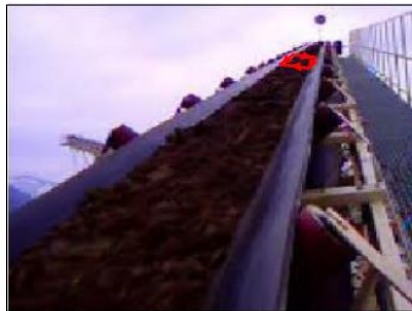
Fig. 1. Determination of the real-time section of the conveyed material using inspection camera
