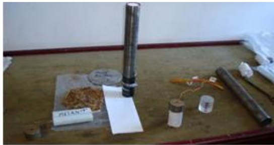
Fig. 3 Preparing confined explosives charge and installing booster and detonator
