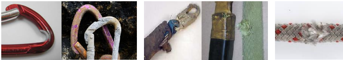
Fig. 1. (a) damaged connectors; (b) damaged energy absorbers and webbing; (c) damaged rope
