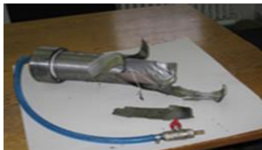
Fig.4 Scrap and shrapnel generated by pipe when testing an explosive gel - 200g cartridge conditioned to hydrostatic pressure
