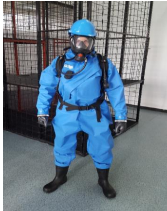
Fig. 1. Chemical protective equipment with breathing apparatus worn on the outside protective suit
