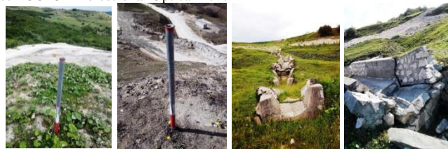
Fig. 2 (a) and (b) 3D tracking points; (c) and (d) Deformations/ effects on Plaiul Cheii hill
