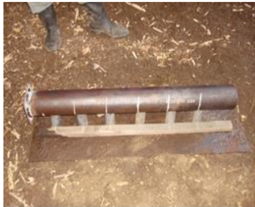
Fig. 2 Confined explosive charge in steel pipe prepared in blast bunker
