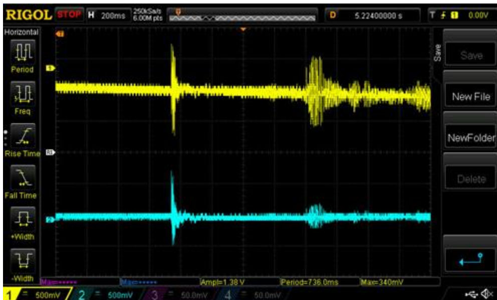
Fig. 1. Measurement of explosion pressure in blast bunker with two piezoelectric transducers - catch oscilloscope image
