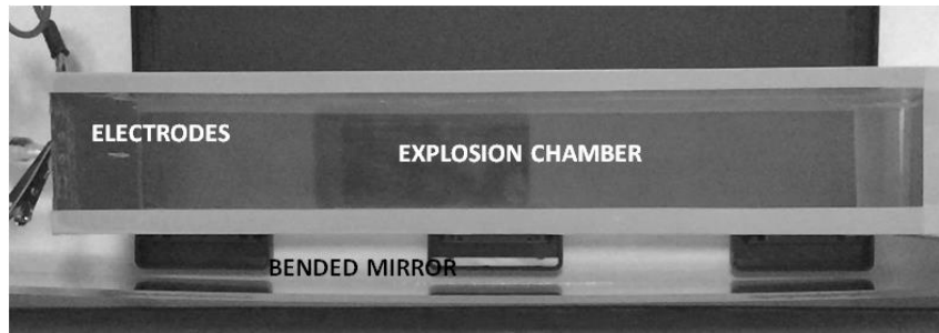
Figure 3. The transparent explosion chamber and the bended mirror (top view)
