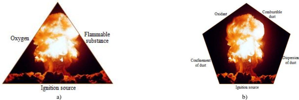
Fig. 1. (a) explosion triangle; (b) explosion pentagon
