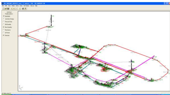
Fig. 3. Uricani ventilation network - VENTEX simulation – 6 bar
