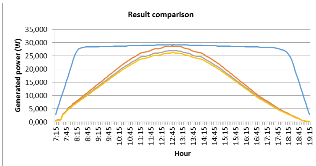
Fig. 4. The values recorded at different inclinations of solar panel during the day
